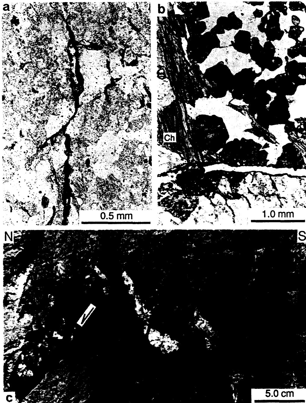
Fig. 2. Fractures and slip surfaces in retrograded gneisses. (a) Intersecting chlorite-filled transgranular fractures in felsic gneiss composed of quartz (white) and clouded plagioclase (light gray) (plane light). (b) Chlorite replacement of garnet (arrow) adjacent to chlorite-filled fractures (horizontal); dilation across fracture near bottom of photograph occurred during thin section preparation (plane light). (c) Zone of fractures and anastomosing chloritic slip surfaces offsetting small granitic dikes in chlorite-rich gneiss; outcrop is located along Animas River approximately 5 km north of northern edge of Fig. 1(c), outside of immediate study area.
